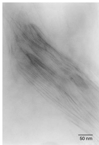
Figure 10. TEM micrograph taken from a silicate particle in a PP/OMMT/MAPP nanocomposite. See the loose structure, changing platelet density and individual platelets
