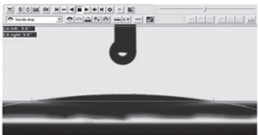
Figure 4. Measurement of the contact angle in OCA software
