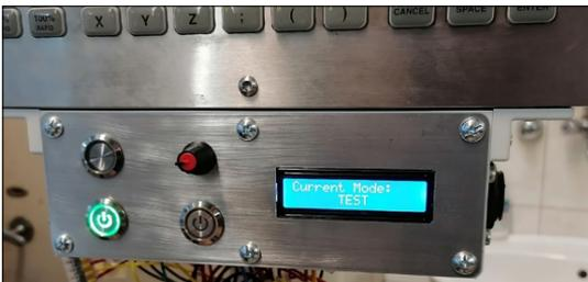
**Fig. 11.** Enclosures for laser head control electronics.
