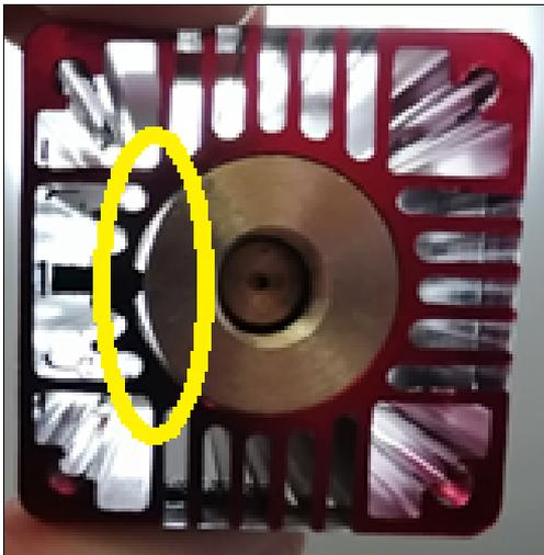
Fig. 4. Factory Cooling System Failure of the Laser Module.
