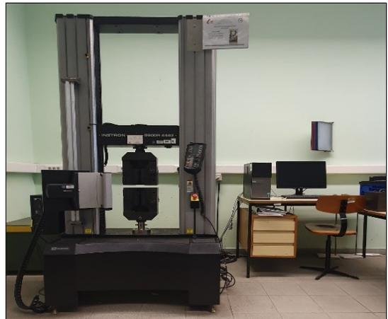
**Fig. 1.** Instron4482 electromechanical universal testing machine.
