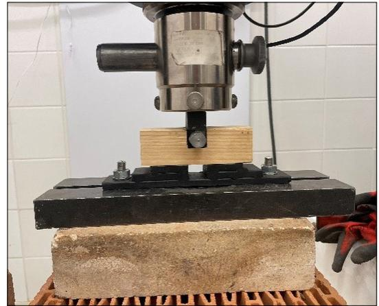
**Fig. 19.** Shear load test with weakening.
