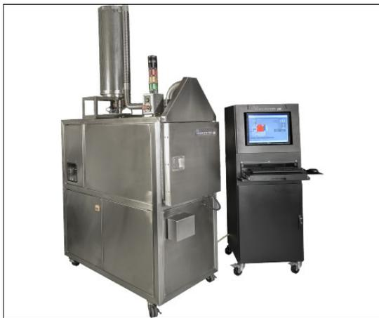
**Fig. 4.** CD 3045 binder removal furnace. [18]
