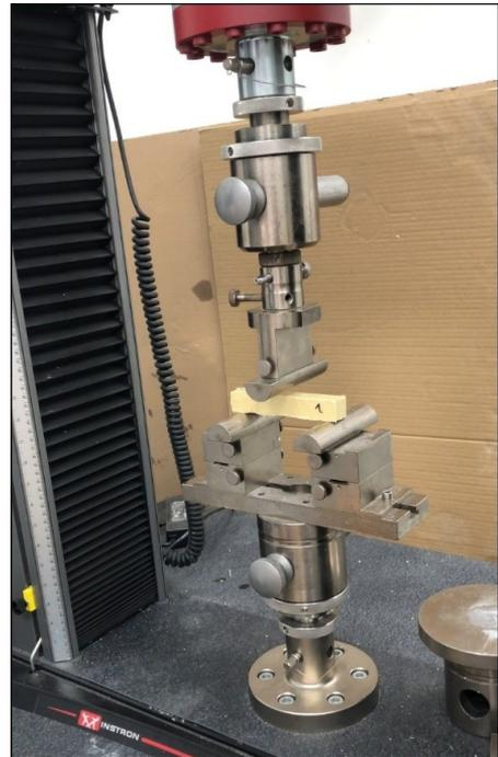
**Fig. 8.** Resin specimen tested for bending.
