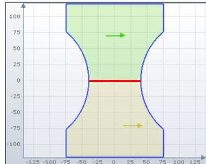
**Fig. 6.** Location of weld seam, type ‚B‘
