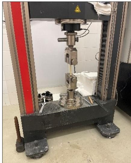
**Fig. 3.** Measurement of tensile strength of resin.
