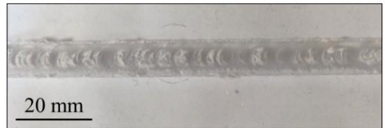
Fig. 8. A characteristic seam from a top view.
