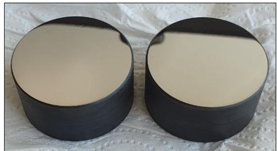
**Fig. 2.** The polished pressure plates.
