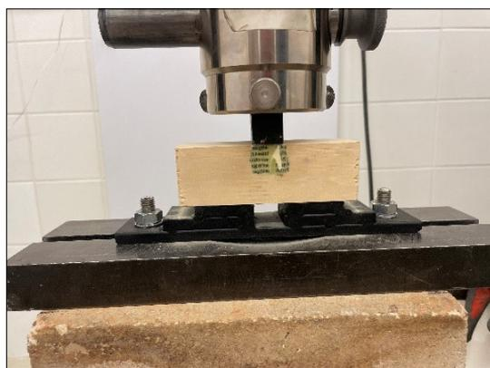
Fig. 21. Shear test specimens supplemented with resins.
