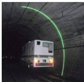
(a) A inspection vehicle for normal-speed railway tunnels
