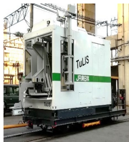
(b) A inspection vehicle for Shinkansen tunnels put into use in 2020
