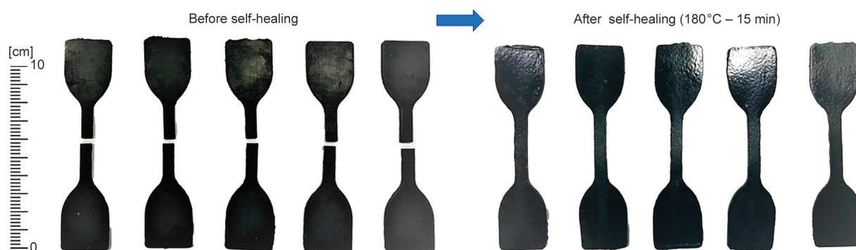
Figure 4. Representative pictures – original tensile-fractured samples before self-healing and after self-healing at 180 °C for 15 min.
