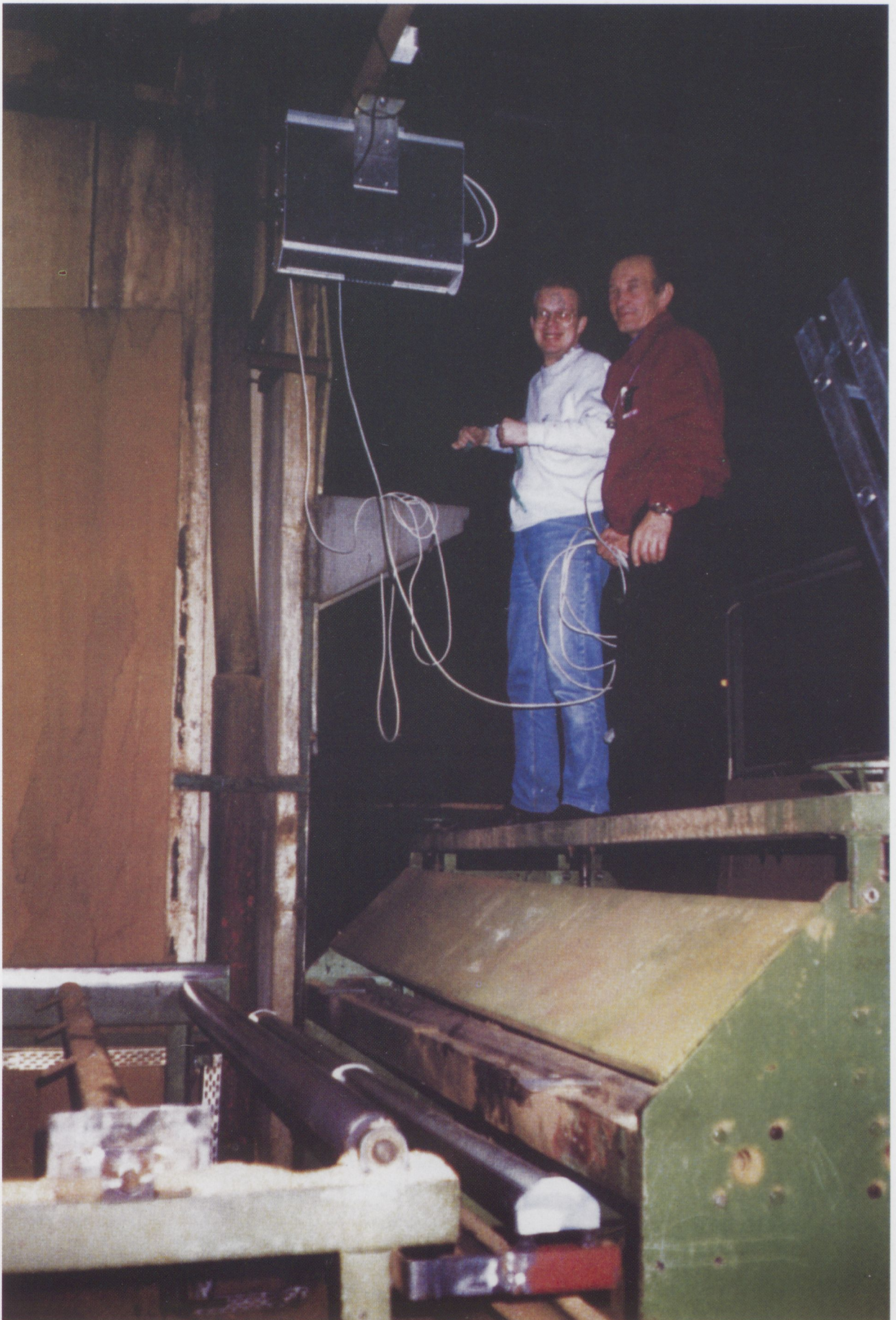
Fig. 25. Mounting of the microwave monitoring system at the particleboard plant.
