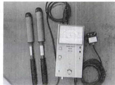
Fig. 8. Photograph of the power density meter
