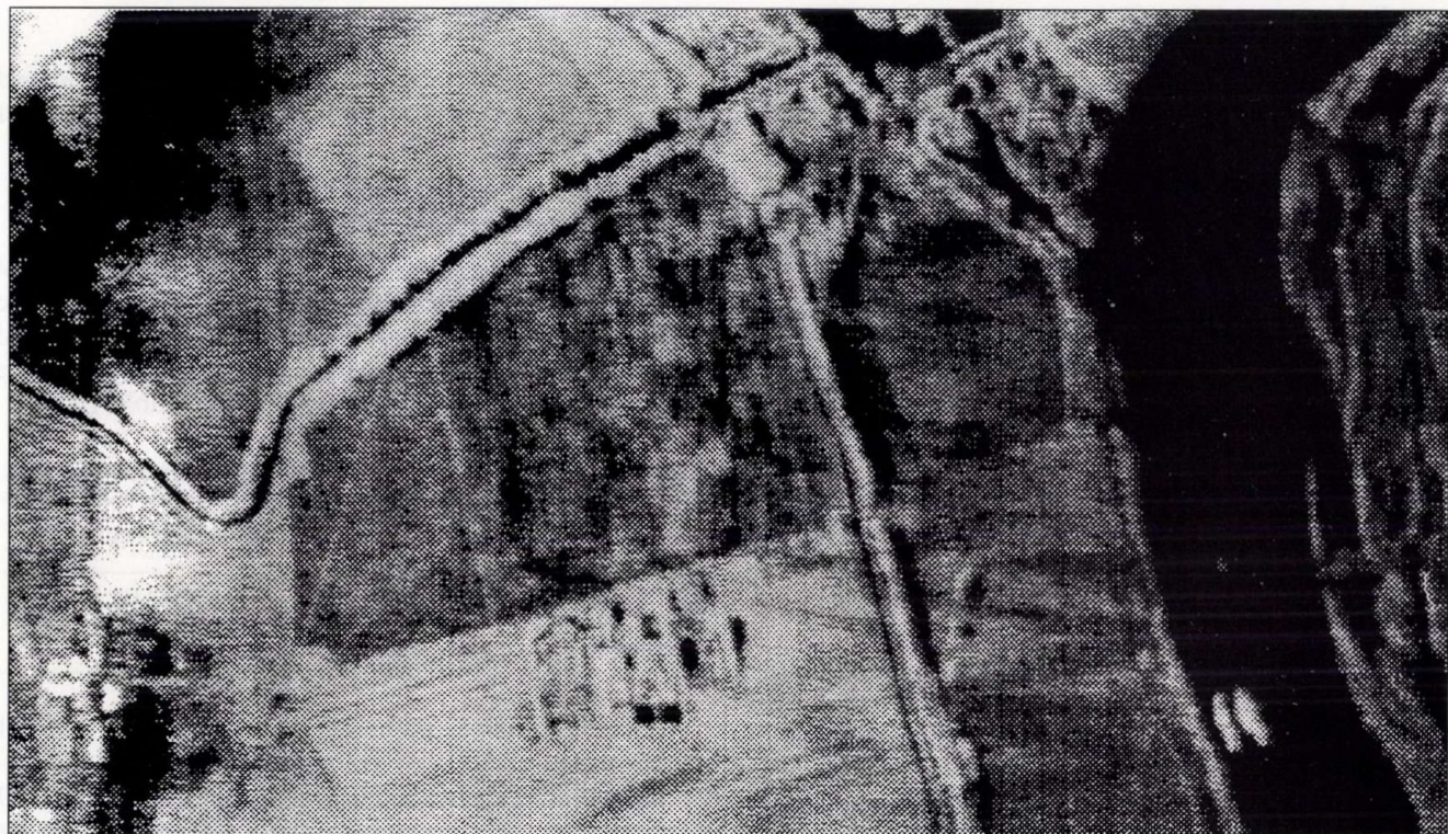
Fig. 5. SLAR image after average correction for near-range showing river Danube (right) and agricultural fields with roads (left)
