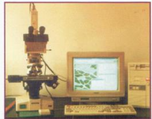
Proprietary image analysis system - VIRGINIA for morphological studies in materials science and biomedicine.
