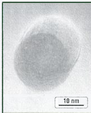
HRTEM image of CN x film deposited onto NaCl substrate at 0.1 mbar partial pressure of N 2 at ambient temperature
