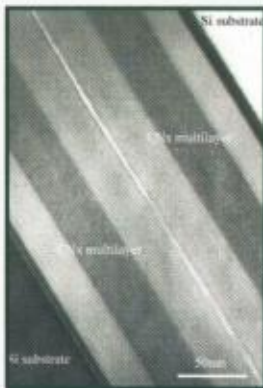
Cross sectional TEM image of a CN x multilayer. Cooperating partner: Forschungsinstitut Rossendorf
