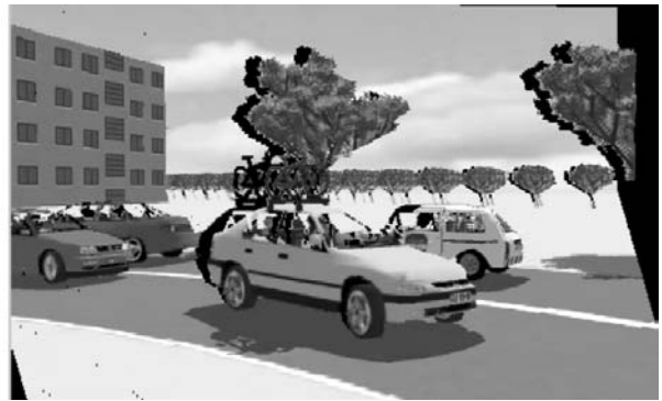
Figure 8/b. Prediction from the nearest right reference image (PSNR = 27.63 dB)
