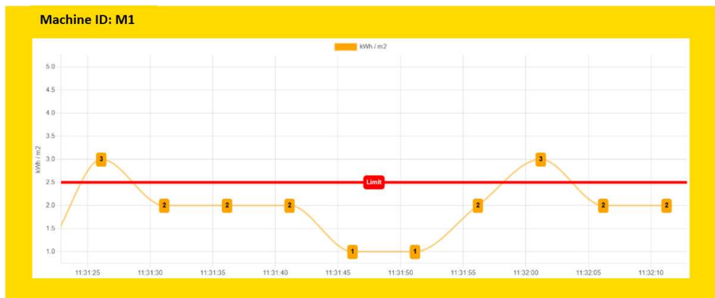
Figure 28. The latest ratio shows wasteful operation (below limit)
