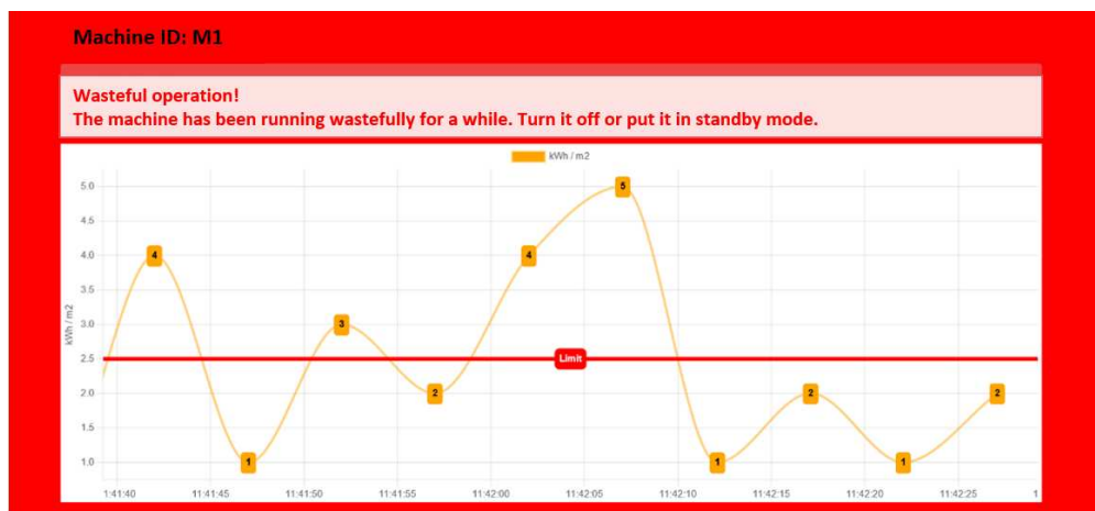
Figure 29. Indication of prolonged wasteful operation
