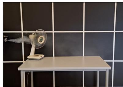
**Fig. 15.** Smoke test of the desk fan.
