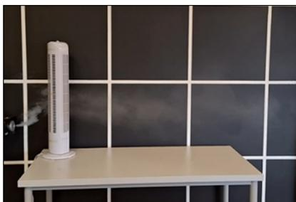
**Fig. 13.** Smoke test of the tower fan.
