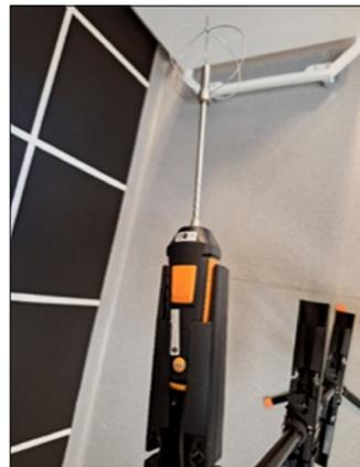
Fig. 8. Testo turbulence probe
