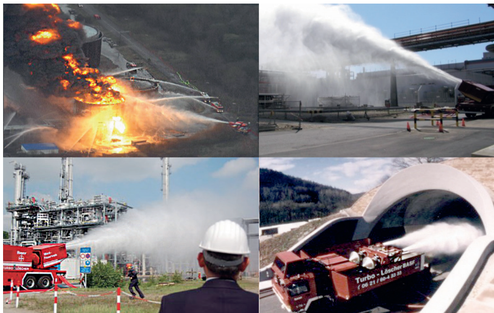
Figure 8: Application possibilities of turbo-reactive extinguishers
