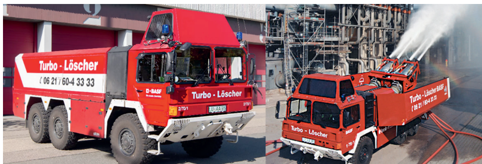
Figure 6: Turbo-reactive extinguisher applied in 1996 by BASF Forrás: BASF 2023
