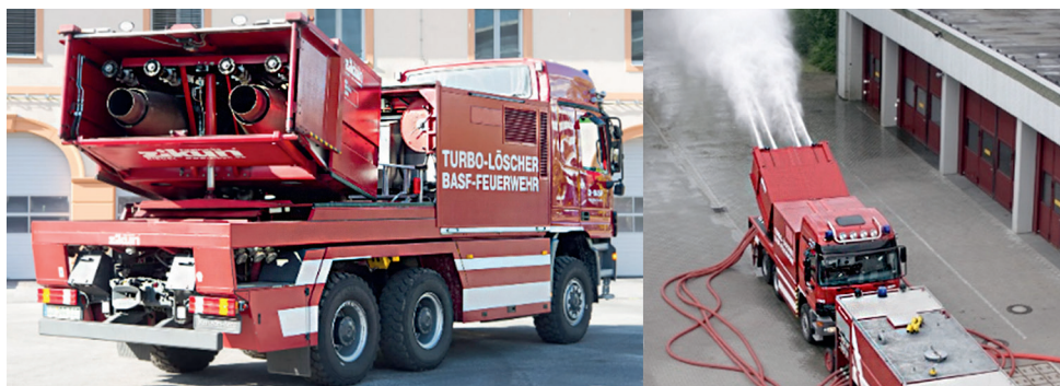
Figure 7: Turbo-reactive extinguisher applied in 2005 by BASF
