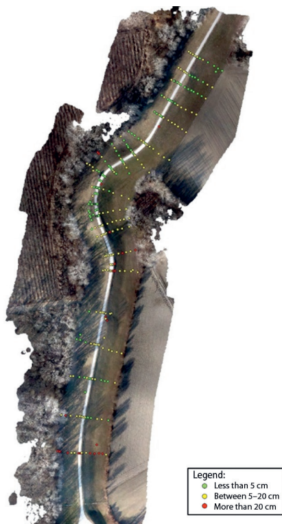
Figure 3: Height differences of orthophoto points
