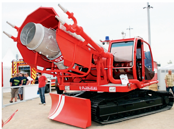
Figure 2: Turbo-reactive extinguisher manufactured by Russian Pozhtekhnika
