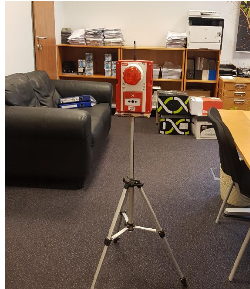
Figure 5. Used fire alarm sounder, source: own photo
