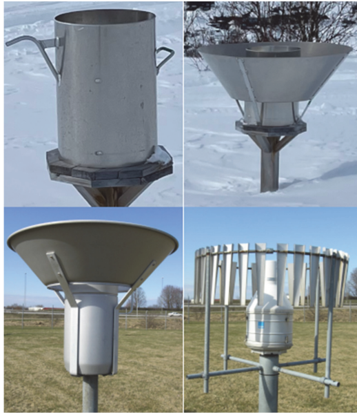
Fig. 1. The four precipitation gauges included in this study, the historical unshielded gauge (top left), the historical shielded gauge (top right), the modern manually operated SMHI-gauge (bottom left), and the GEONOR automatic gauge (bottom right).
