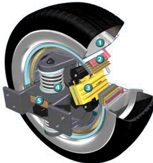
Figure 8: Siemens VDO eCorner, wheel rim (1); wheel hub motor (2); electronic wedge brake (3); suspension (4); electronic steering (5). Source: Siemens VDO Automotive AG, (Gerling, Dajaku and Lange, 2007)
