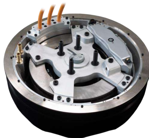
Figure 12: Elaphe L1500 radial flux IWM (Gallery - Elaphe, 2024).
