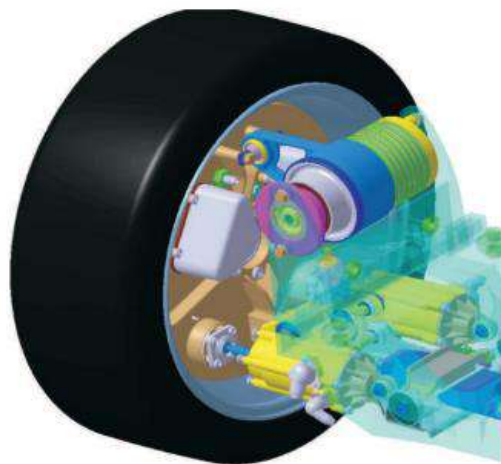
Figure 5: Schematic diagram of Volvo's Autonomous Corner Module, (Jonasson, Zetterström and Stensson Trigell, 2006).
