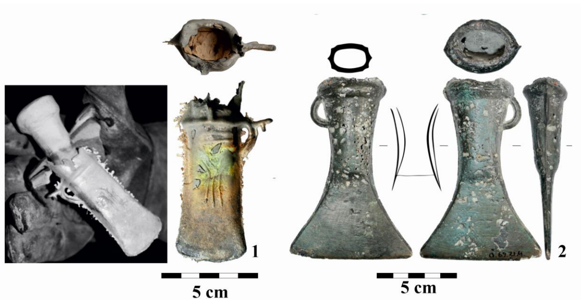
Fig. 9.: Core rising defects: 9/1: Experimental socketed axe; 9/2: A socketed axe with core rising defect from Beremend (modified after Tarbay 2018, Pl. 256.4).
