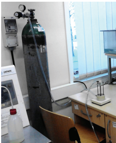
Figure 12. Nitrogen bottle connected to pressure regulator and linked to flow meter.
