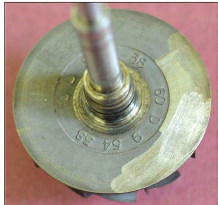
**Figure 5.** Wear traces on the turbine wheel.
