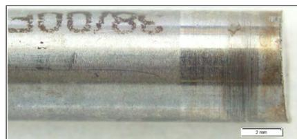
**Figure 6.** Wear marks on the shaft.
