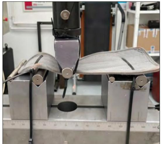
**Figure 4.** The orthosis in the apparatus designed for fatigue testing.
