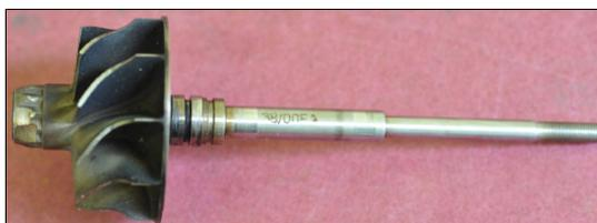
**Figure 4.** The welded turbine and shaft.
