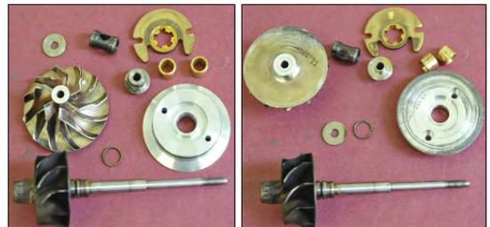
**Figure 1.** Parts of the internal assembly of the failed turbocharger; the total length of the turbine + shaft assembly is 120 mm.
