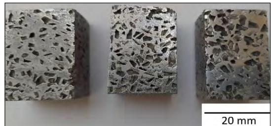
**Figure 2.** Picture of the specimens (from left to right open cell meta foam with Al<sub>2</sub>O<sub>3</sub> reinforcement, Reinforcement metal foam by SiC and unreinforcement open cell metal foam.
