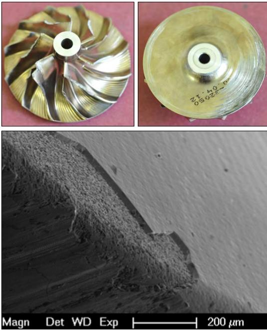
**Figure 12.** Wear marks on the compressor wheel.
