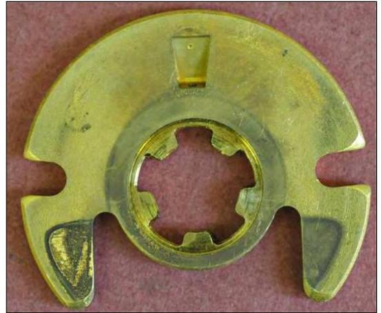
**Figure 10.** Wear marks on the axial bearing.
