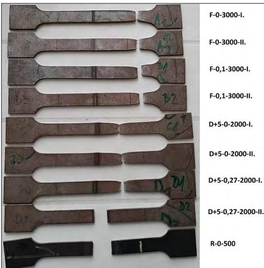
**Figure 6.** Tensile test specimens.
