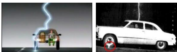
Figure 6: Lightning current route in schematic diagram and in reality [12][13]
