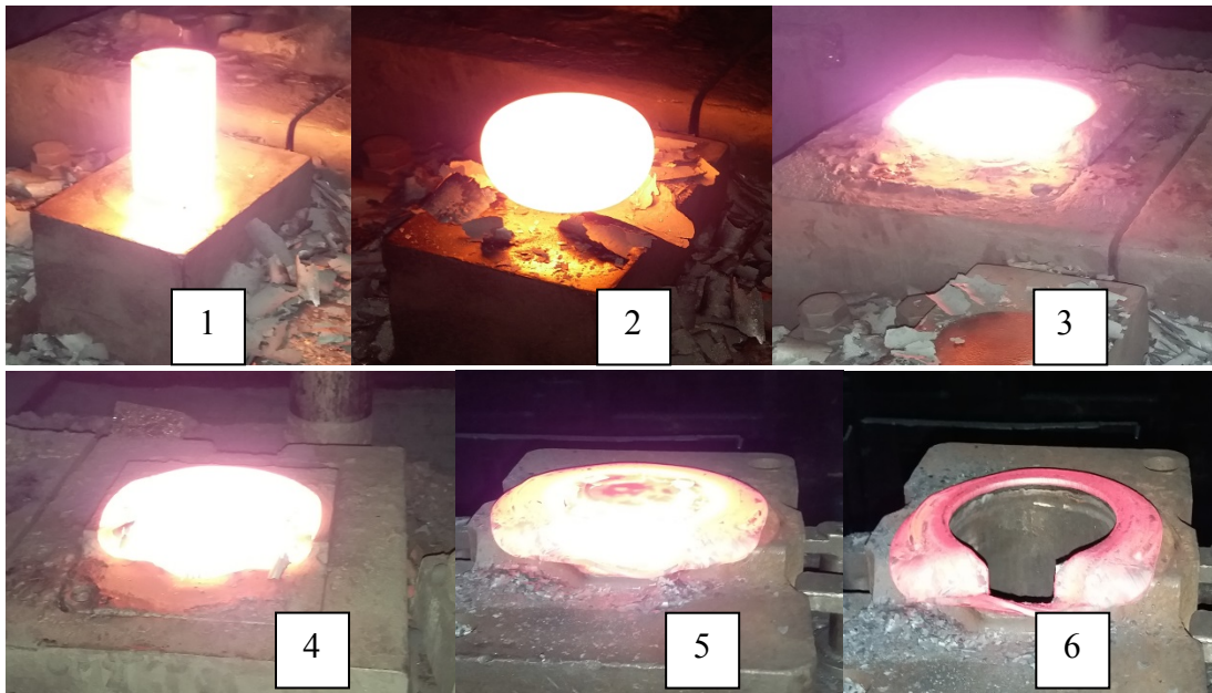
1. Figure: Forging steps
