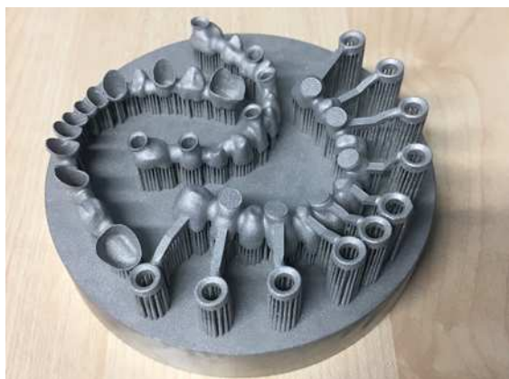
Fig.15. Printed, heat-treated, sandblasted platform
