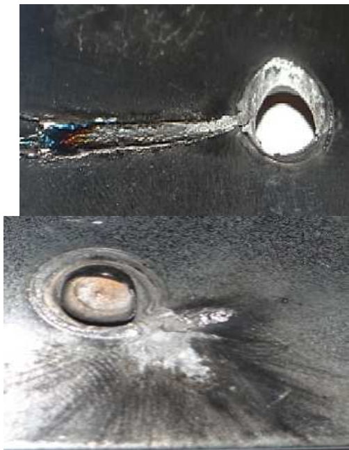
Fig. 7: Expulsion trace in the DP00/ X8Cr17 RSW.
