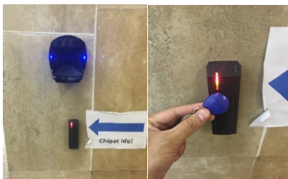
Figure 3: The proximity device (Tag)
