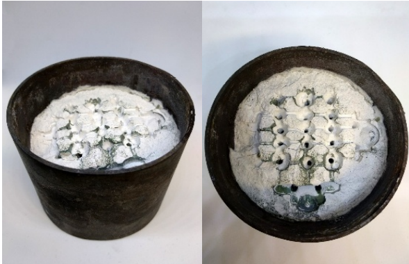
Fig. 5: Cracked embedding material
