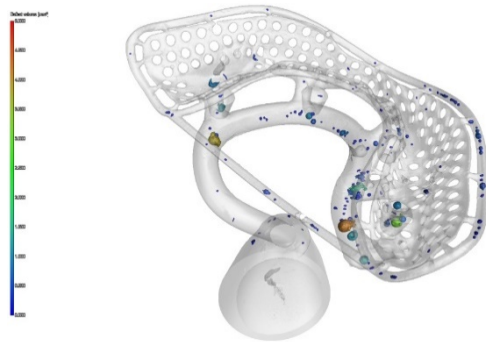
Fig. 9 b): Inclusions can be detected by CT imaging
