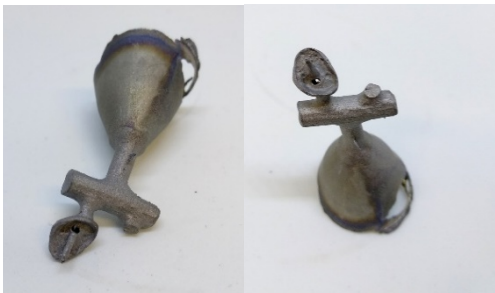
Fig. 6: Workpiece with argon gas generated casting cavities
