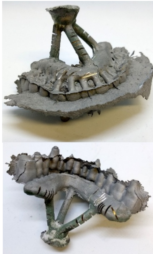
Fig. 7: A defect originating from the cracking of the embedding material
