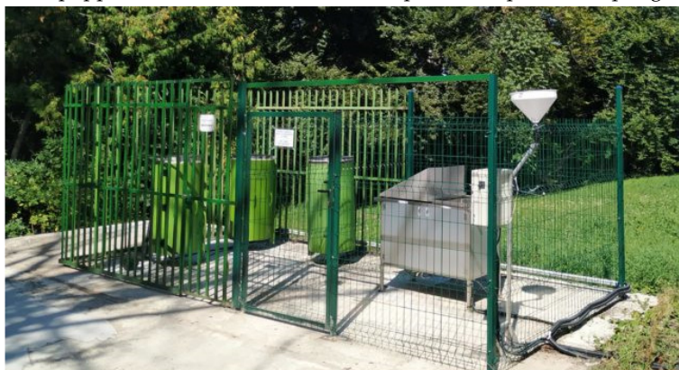
Figure 7: Radioactive deposition collectors at Station 1 of the environmental radiological monitoring system operated at the KFKI Campus – collectors used in parallel for combined deposition sampling (on the left), and collector for separate sampling of wet and dry deposition (on the right)
