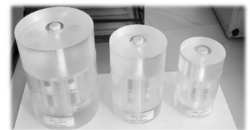
Figure 1: Thyroid phantoms: ANSI (above); SURO (below).
