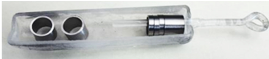
Figure 1: Ring samples prepared for thermal treatment in inert atmosphere
