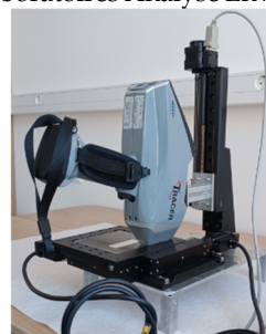
Figure 1: The new Bruker portable X-ray fluorescence spectrometer and the xyz sample stage
