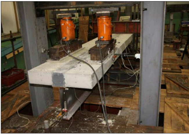
Fig. 5: Steel concrete composite beam with the UHPC joint of the precast slab – scheme of the test
