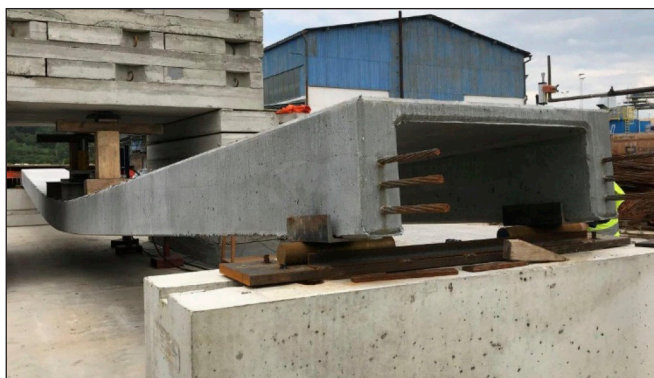
Fig. 11: Loading test of a pretensioned beam
