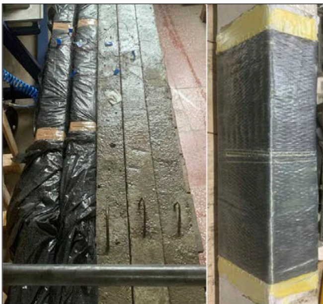
Fig. 5: Beams before testing with some still wrapped in plastic (left) CFRP wrapping on beam 7 (right)
