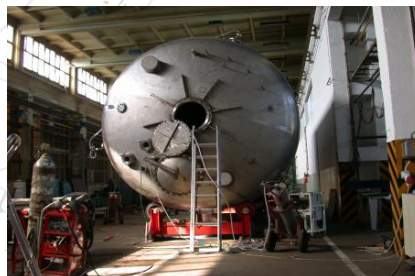
On-site special leak testing
