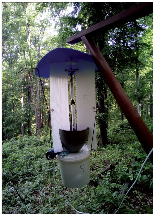
Fig. 2: The light trap used for sampling with a UV tube and battery
