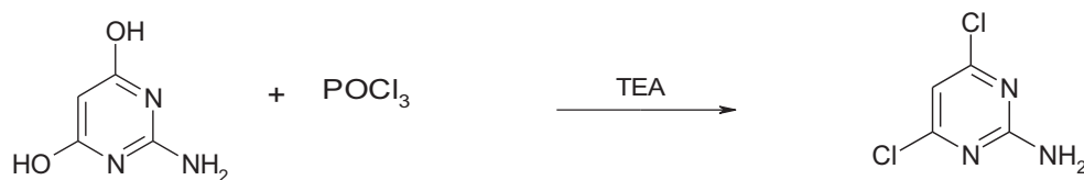
Figure 2 Formation of 2-amino-4,6-dichloropyrimidine (ADCP) using phosphorous-oxychloride
