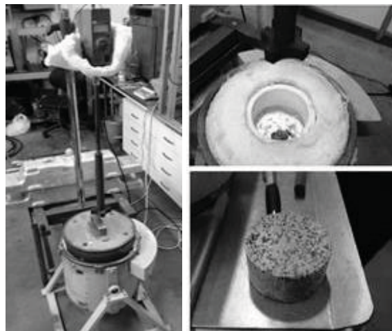
Figure 2 The smelting-holding furnace used for the experiments
