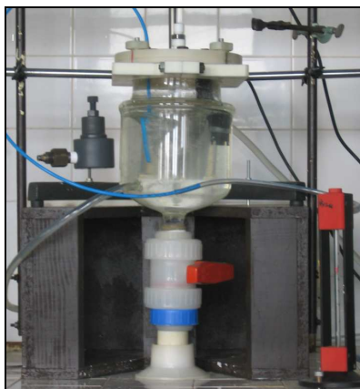
Figure 6. The home-made precipitation reactor assembled at the Department of Non-Ferrous Metallurgy at University of Miskolc
