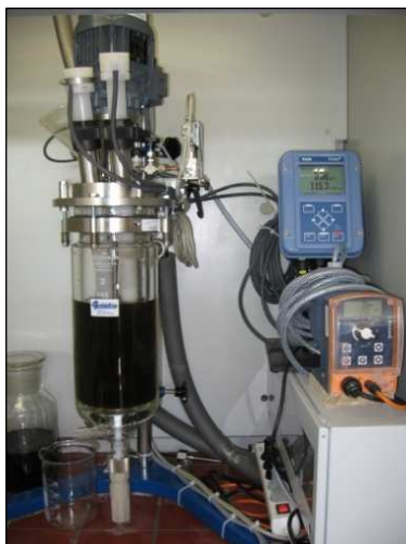
Figure 1. Photograph of the precipitation apparatus equipped with a mechanical stirrer, a CO 2 gas supply unit, and sensors to measure the solution conductivity, pH and temperature
