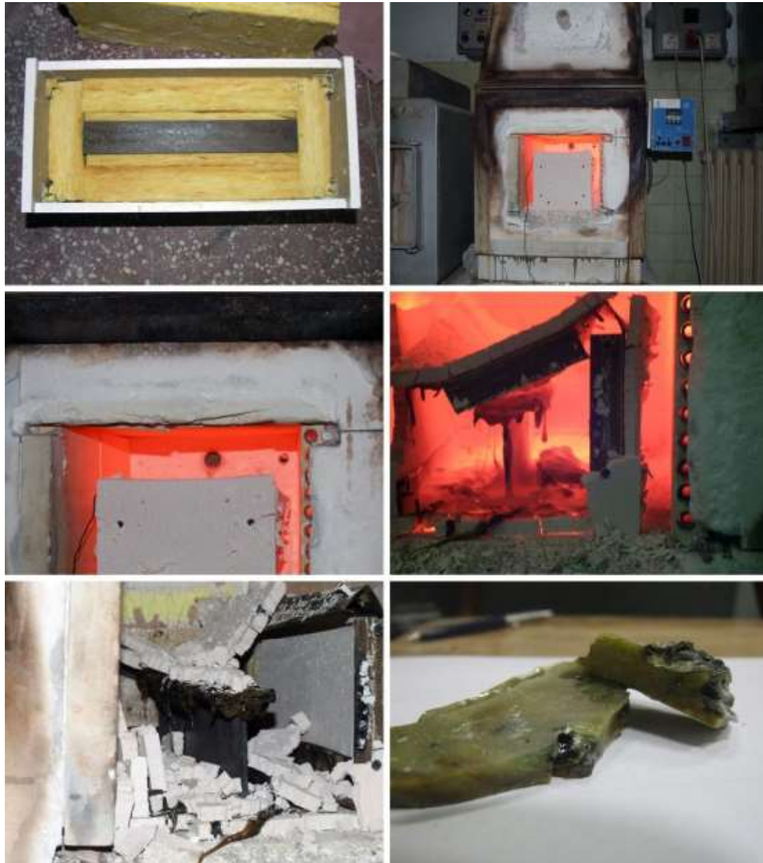
Figure 3- Typical failure of fiberglass insulation.
