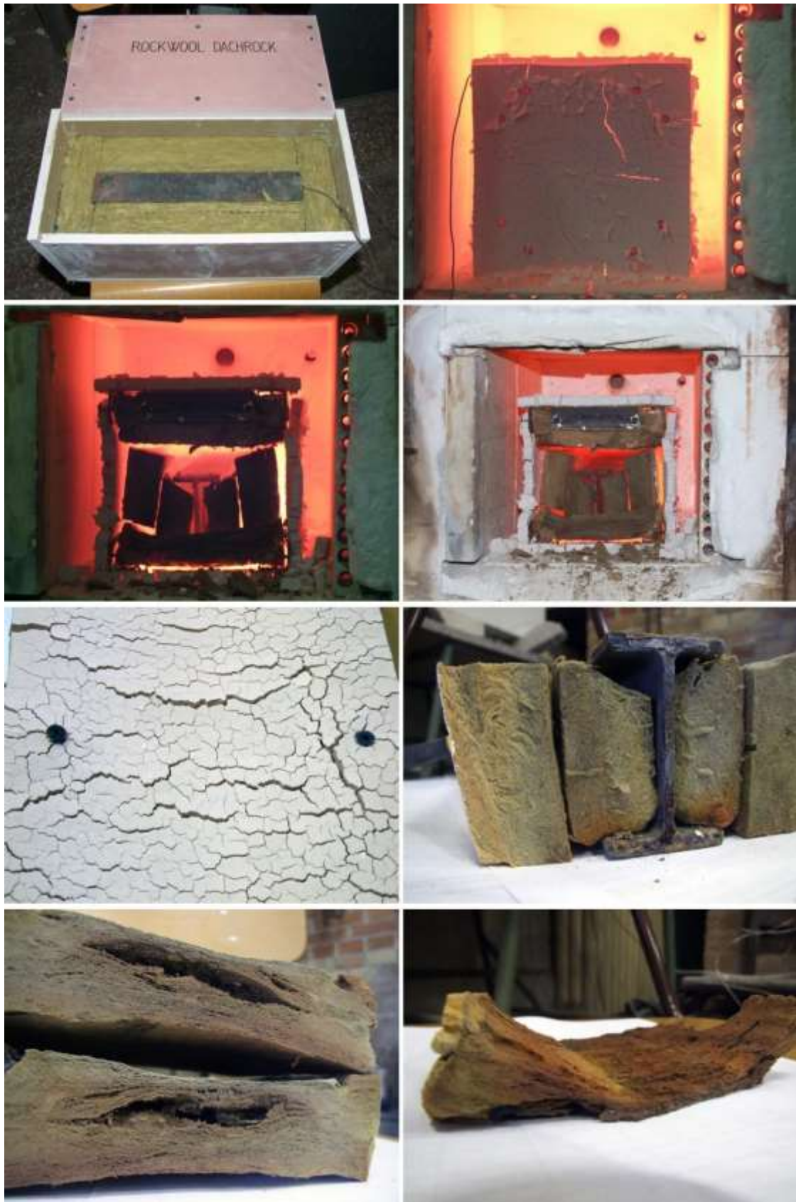
Figure 5- Typical failure of rock wool insulation.
