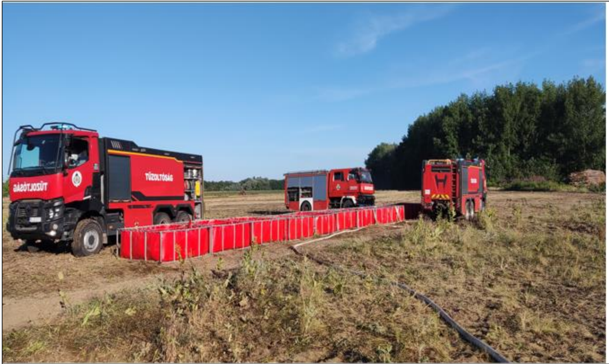
Figure 22.: Two S10 water conveyors and mobile extinguishing water basins (made by the author)
