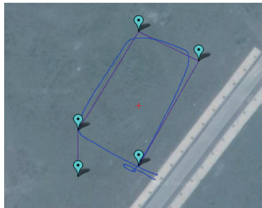
Figure 3. Blue line – real trajectory/Purple line – requested trajectory [21]
