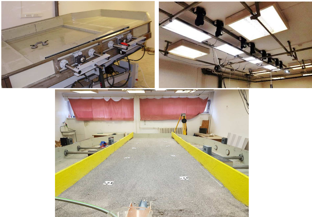
Figure 2. Images depicting the PTHETHYS flume's construction: (A) View of the PTETHYS flume before installation; (B) The series of cameras installed for recording geomorphic processes; (C) A prepared flume prior to the start of an experiment
