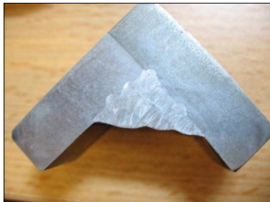
Figure 3. Welded joint, polished and etched.
