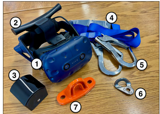
Figure 1. Tools used in the research: (1) HTC Vive PRO VR glasses, (2) VIVE Wireless Adapter, (3) SteamVR Base Station 2.0, (4) Portwest FP51 Y sling, (5) Portwest FP35 hook carabiner, (6) CADO AT 150 fixed mooring point, (7) CADO AT 150 fixed mooring point.
