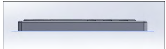
Figure 6. Side view of the parting plane (marked with a blue line at the bottom of the part).
