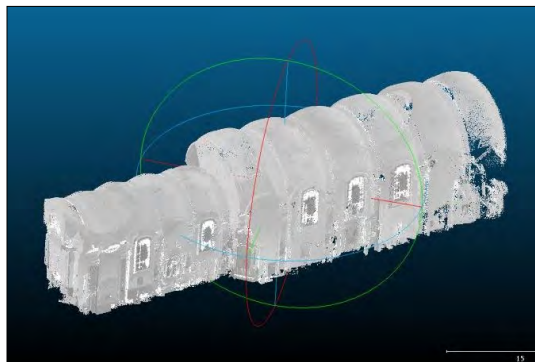
Figure 4. A three-dimensional model created by merging the points recorded with the scanner into a point cloud.
