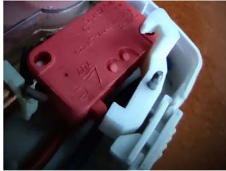
Figure 4. 3D printed switch arm being installed
