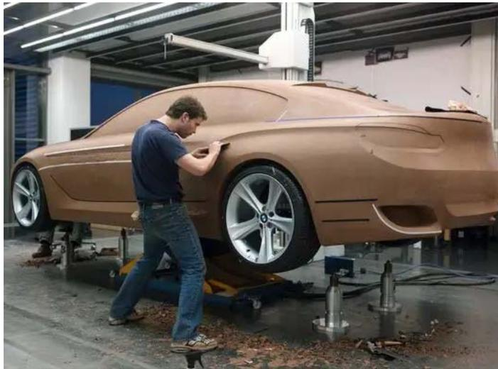
*Figure 3 Creating a car body clay model [F3]*
