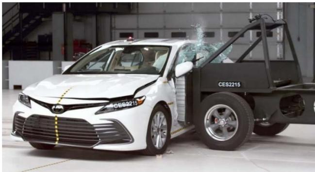
*Figure 6 Side impact test [F6]*
