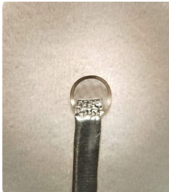
Figure 3. Electron microscopy nickel grid (300 mesh) with aluminium foil handle for vitrification of oocytes
