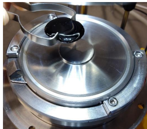
Figure 3. Putting a 25 mm diameter specimen onto the DSR plate
