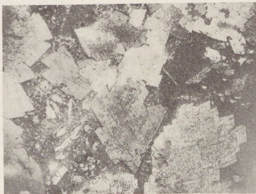
Fig. 6. Idiomorphic calcite and manganocalcite crystals in the submicroscopic ankeritic and silicic ground mass. Parallel nicols, 25 x.
