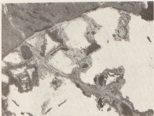
Fig. 2. \text{FeS}_2 -I. generation, idiomorphic crystals in chalcopyrite. The interior of the chalcopyrite is mottled with fields and veins consisting of \text{Cu}_2\text{S} and \text{CuS} . (white: chalcopyrite, pale grey: pyrite, light grey: chalcocite-covellite, dark grey: manganocalcite. Parallel nicols, 125 x.
