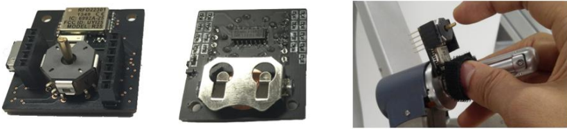
Figure 5: The NMI structure: (a) front side, (b) back side, (c) NMI attached on the MTM.
