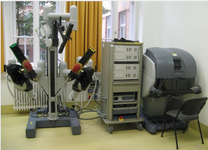
Figure 4: The da Vinci Surgical System and the da Vinci Research kit. System components: Patient Side Manipulators (left), the dVRK controller (middle) and the Master Tool Manipulators (right).
