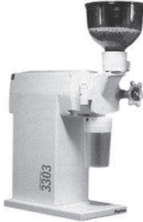
Figure 2: Perten 3303 laboratory mill
