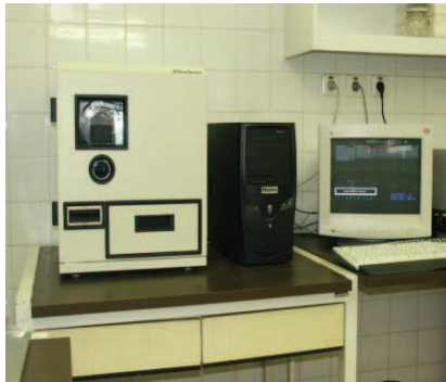
Figure 1: Perten SKCS 4100 instrument
