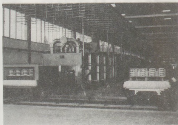
Fig. 5 Fast firing kiln table conveyance (length on average: 70m, output: approx. 10 t/24 h)
