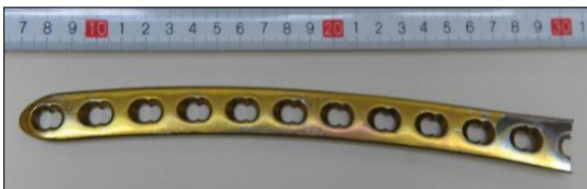
Figure 2. Distal part of the broken bone fixation plate.
