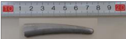
Figure 1. The distal part of the broken hip implant.
