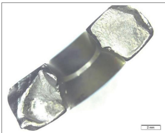
Figure 5. Stereomicroscopic image of the fracture surfaces of the bone fixation plate.
