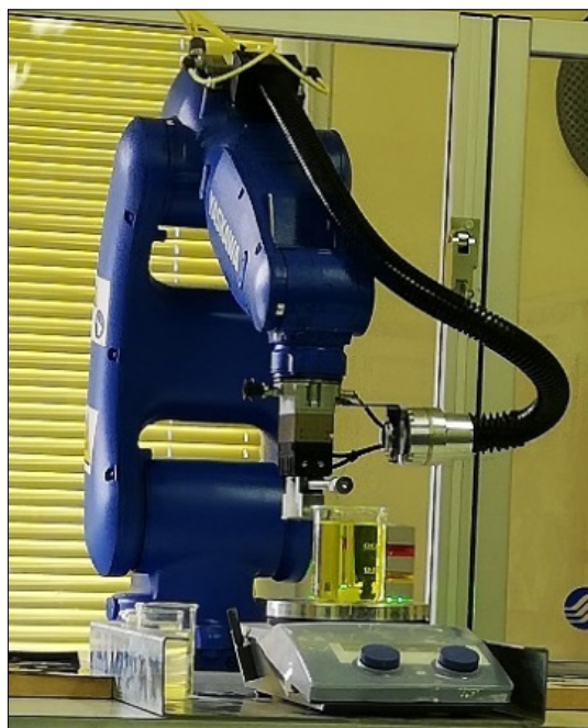
Figure 2. Surface treatment with a Yaskawa „You teach me” robotic arm.
