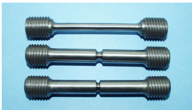
Figure 3 Characteristics of the un-notched and notched specimens
