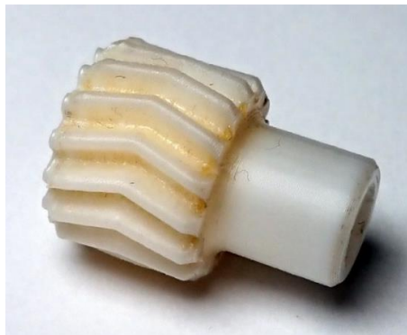
Figure 9. The input sun gear after more than 300,000 revolutions
