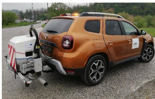
Figure 3. Test vehicle with built-in measuring equipment
