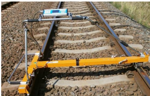
Figure 1. Electronic self-recording track gauge TEC-1435 N2
