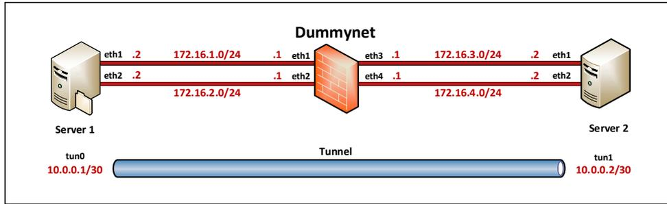
Figure 5. Our new measurement testbed with Dummynet.
