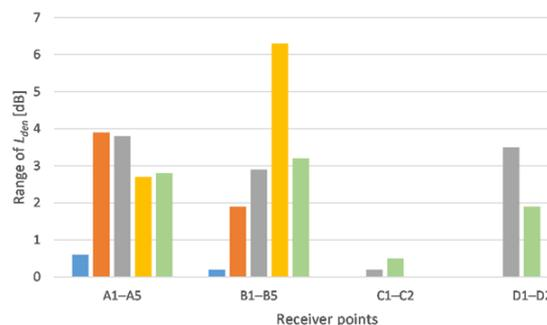
**Figure 4.** Maximum differences in day-evening-night sound levels (Lden) in dB for the test cases at each receiver point
